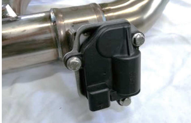
Fig. 5 Installed with stock actuator (photo shows left #2 mid pipe)
