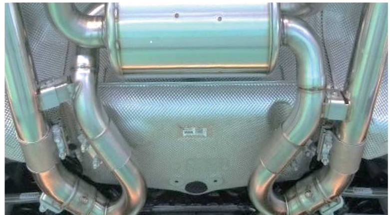
Fig. 16 Detail of main muffler joint
